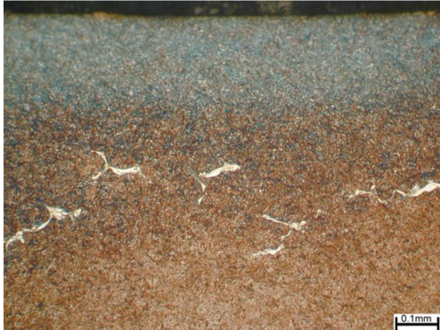
Figure 19 White etching areas around cracks in a rotor bearing from the field [13]
