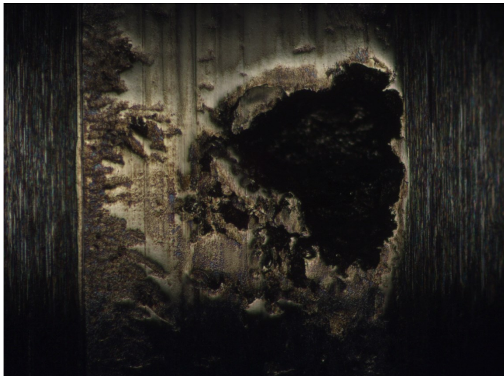
Figure 45 The pitted surface of the roller after 23.3 million cycles in the preliminary test with commercial transmission oil.
