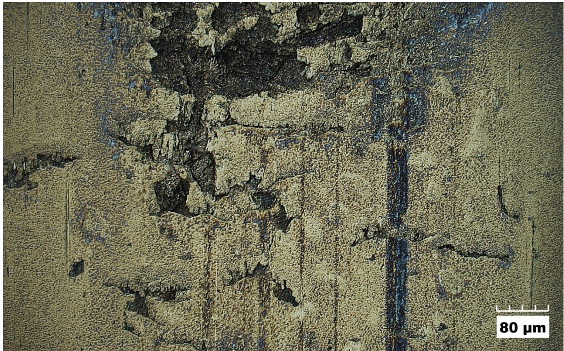
Figure 103 Test 24: surface damage caused by the laser groove on the roller specimen after end of test, 30 million cycles.
