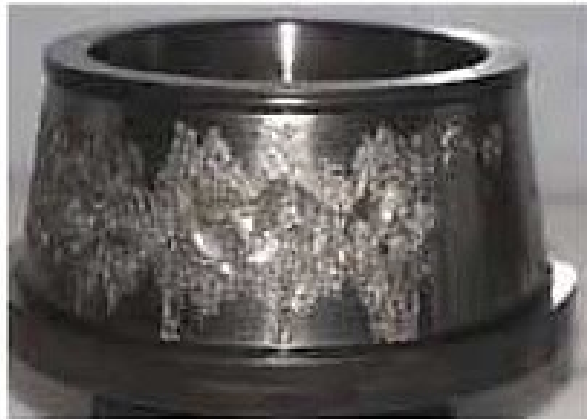
Figure 9 Surface damage on an inner ring of a wind turbine tapered roller bearing [48]
