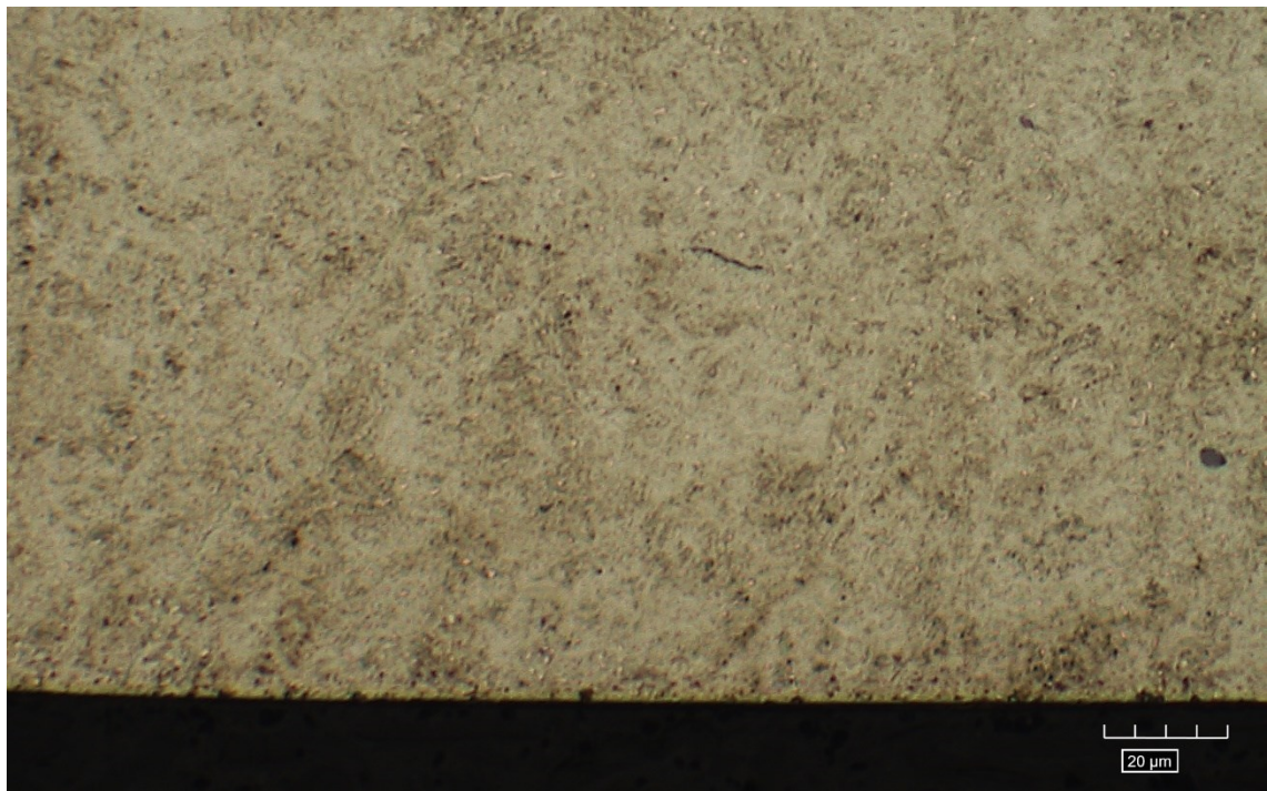
Figure 42 Example optical image of an etched specimen cross-section. The etchant brings in evidence the microstructure of the steel, made of lath martensite, primary and tempered carbides and possible non-metallic inclusions
