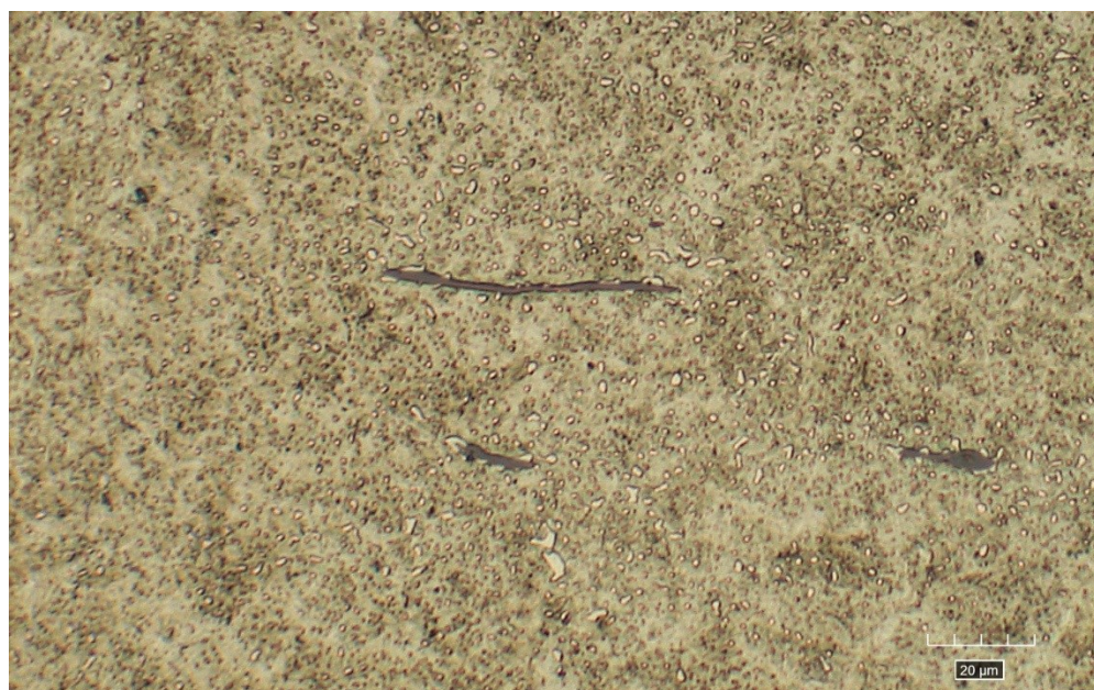
Figure 40 Microstructure of the steel adopted in the present work is shown in a section parallel to the main axis of the roller. Presence of numerous carbides and non-metallic inclusions is reported
