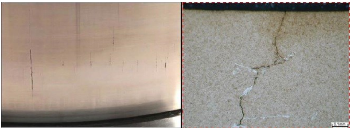
Figure 27 Axial cracks on an inner ring raceway (left) and in circumferential section (right) [13]
