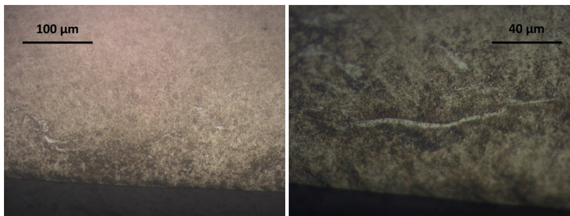
Figure 56 Test 15: WECs observed in the sectioned specimen
