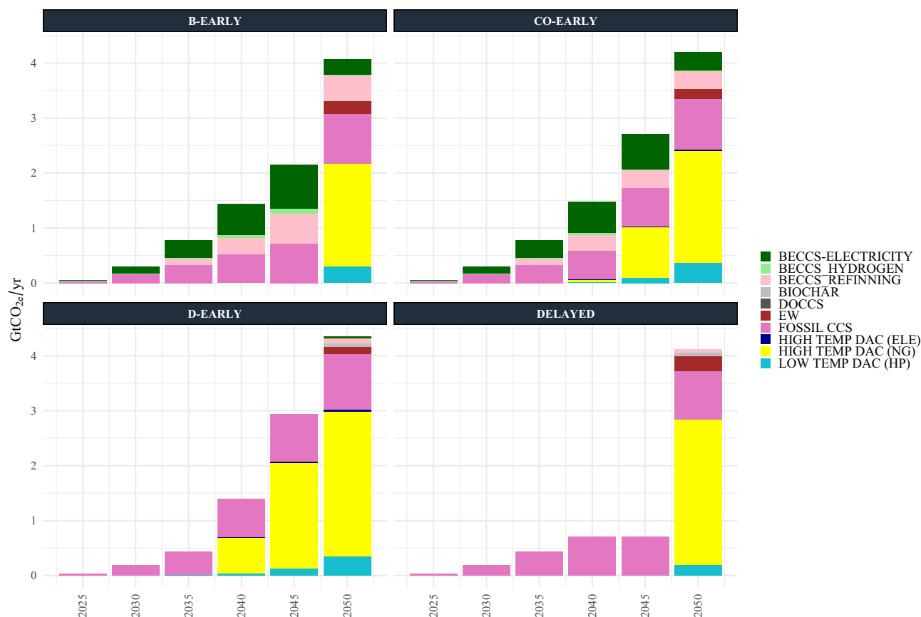
Fig. 6 | Carbon sequestration. Carbon sequestration by technology across the scenarios for near-term CDR deployment and postponement of novel CDR technologies. ELE, NG, and HP represent electricity, natural gas, and heat pumps, respectively, as energy sources for DAC operations.
