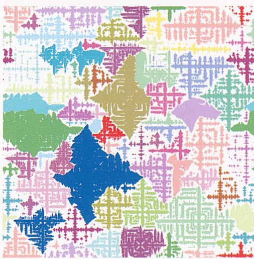
Figure 3-4. Example of the dendrite morphology produced by the solidification model using a 500x500x25 cell domain.
