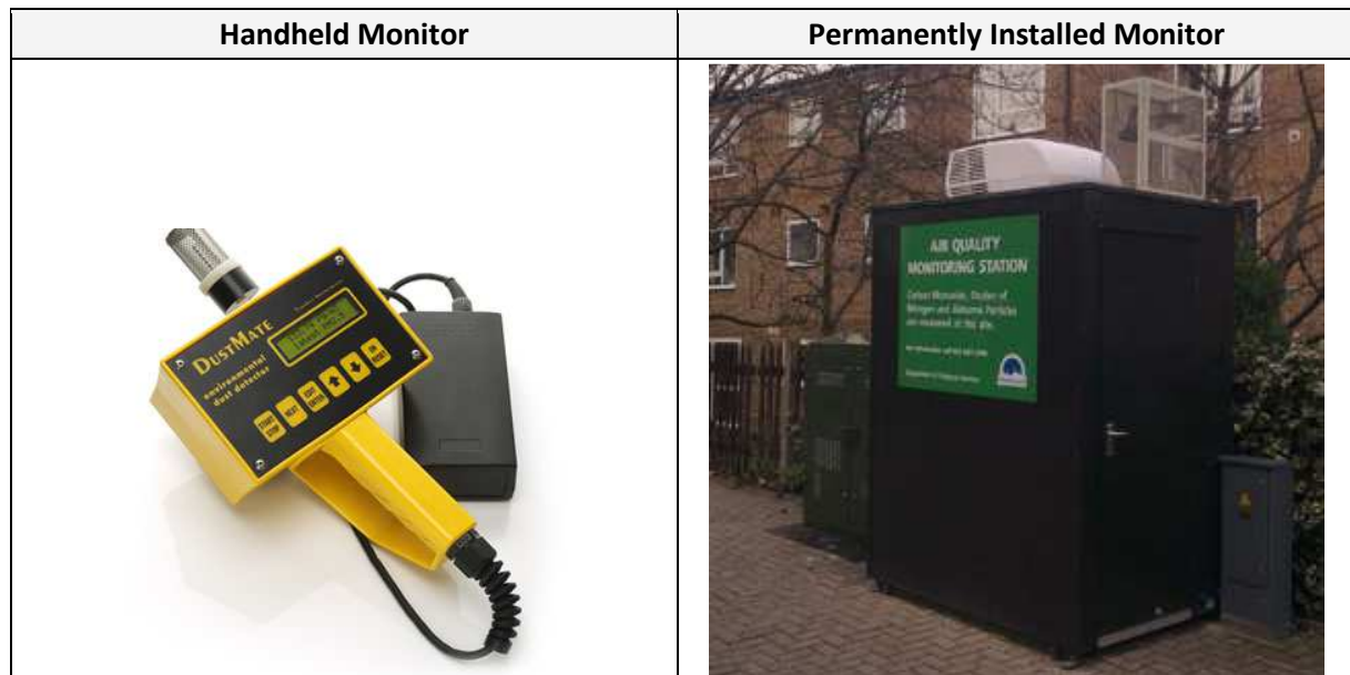
Figure 2: Left side: A handheld Dustmate monitor from Turnkey ( http://www.turnkey-instruments.com , accessed: 11 th Sept. 2013); right side: a permanently installed monitor at a monitoring site in London. Source: London Air Quality Network ( http://www.londonair.org.uk , accessed: 11 th Sept. 2013).
