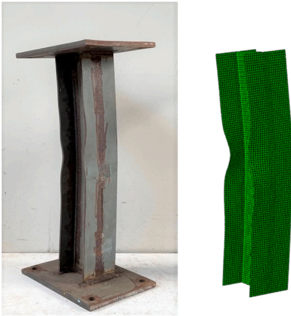
Fig. 8. Comparison of FE and test failure modes for specimen I1-E60.0 [18].
