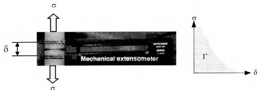
Figure 2.16 Direct determination of the cohesive law using a mechanical extensometer.
