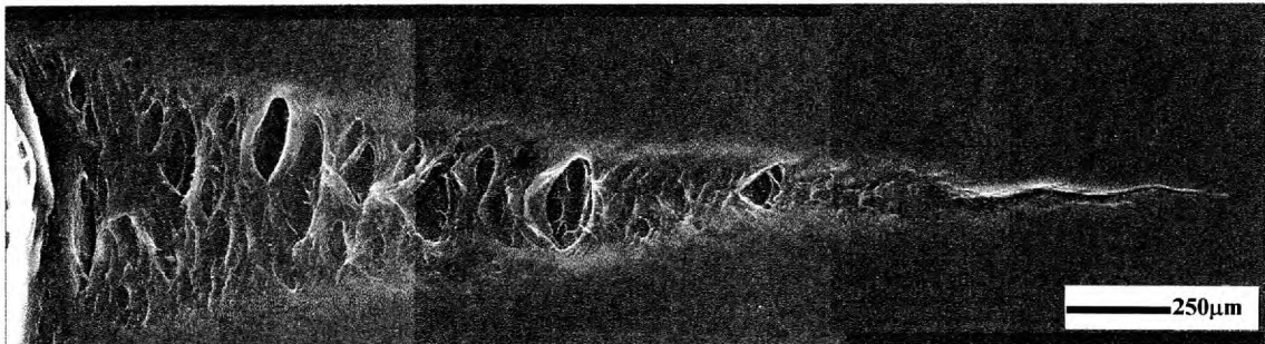
Figure 2.3 A typical craze structure.
