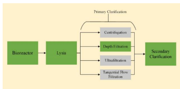
Figure 1: CFPS production process with primary clarification alternatives
