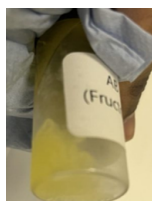
Figure 7: HMF Effluent from Amberlyst-Catalysed Reaction after 24 hours at -70^{\circ}\text{C} . At the top of the vial, a yellow-brown liquid, whilst at the bottom, a solid can be seen covered in the yellow liquid
