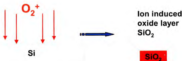
Figure 2.3 Firstly O_2^+ primary ions are implanted into silicon and then an ion induced oxide layer SiO_2 is formed.
