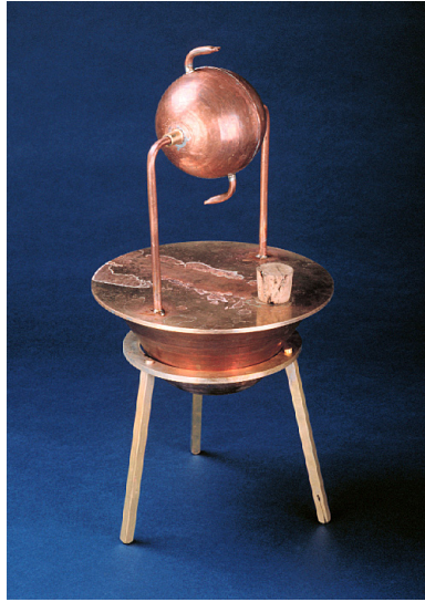
Figure 1.1: A reconstruction of Aeolipile, one of the first known attempts of steam-powered machinery [1].
