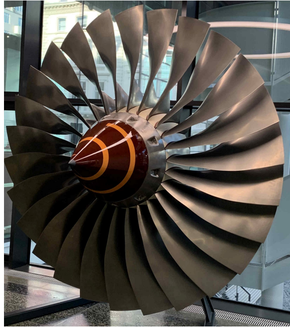
Figure 5.2: A fan assembly of Trent 500 displayed in the Department of Mechanical Engineering at Imperial College London.
