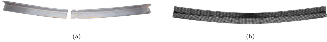
Figure 24: Comparison of deformed beam shape between (a) test and (b) FE model for Specimen 2 ( L = 1000 mm) subjected to major-axis bending.
