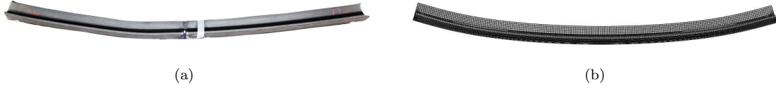
Figure 25: Comparison of deformed beam shape between (a) test and (b) FE model for Specimen 6 ( L = 1000 mm) subjected to minor-axis bending.
