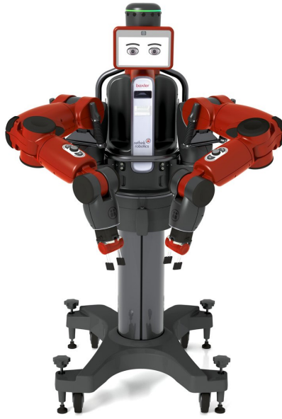
Figure A.1: The Baxter humanoid robot we use for the assistive dressing experiments in this thesis.
