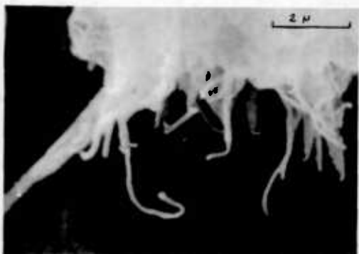
Fig. 90. SEM photograph of same specimen as in fig. 88, showing curved filaments extending from webs.
