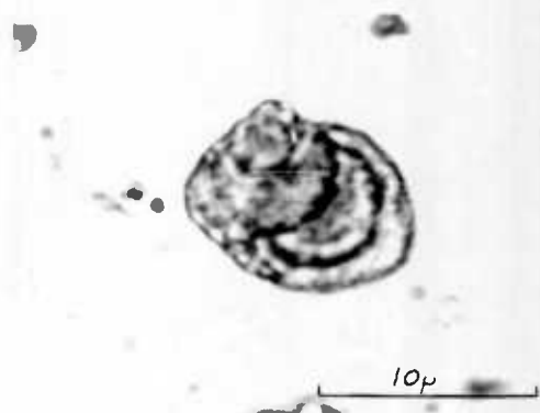
Fig. 75. TLM photograph showing grain with eccentric shell structure. Same sediment as in fig. 73. (SM in PPL.)
