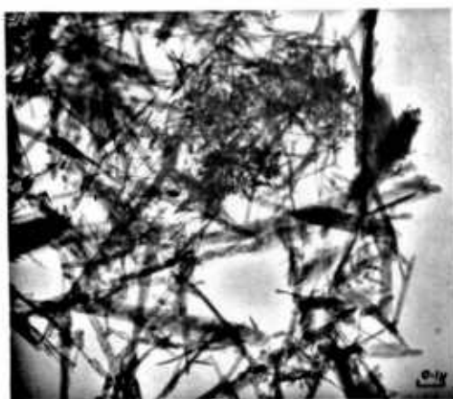
Fig. 101. TEM photograph of same sediment as in fig. 82, showing goethite crystallites of two size ranges and irregular bifurcated filament.
