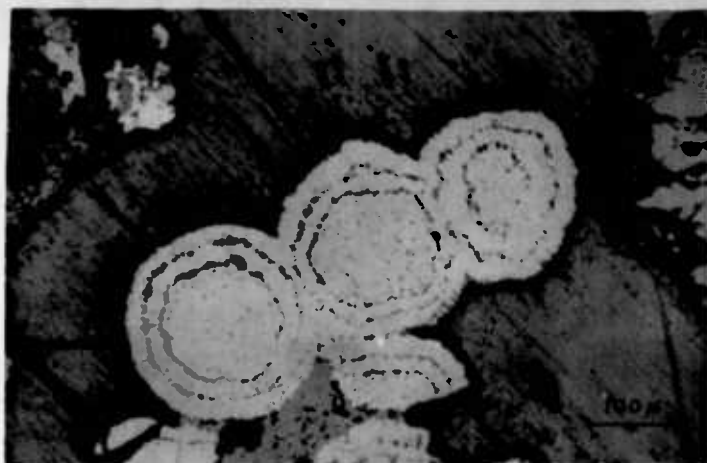
Fig. 27. PLM photograph of zoned spheroidal sphalerite in gypsum from DY19, JJM3, Jabal Dhaylan (PS in PPL).
