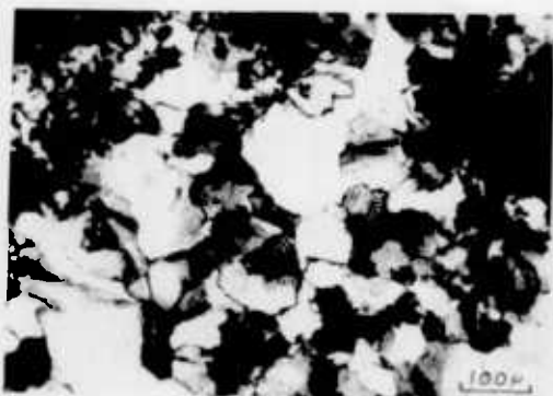
Fig. 131. TLM photograph of Barga jasper showing zoning, patchy extinction and xenomorphic fabric of the quartz (TS in PPL).
