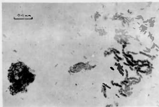
Fig. 109. TLM photograph of maceration residue of Wadi Fatima iron ore showing non-descript algal matter together with cellular tissue or cuticle (SM in PPL).
