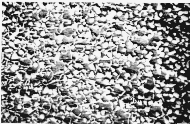
Fig. 57: As-Cast 1 1/2 wt%Si / 5wt % Fe (SEM)
