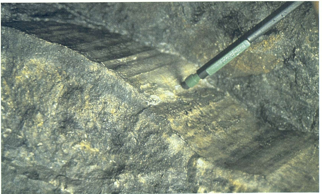
Plate 2.11 Well developed slickensides on the slip surfaces within the Rusey Breccia
