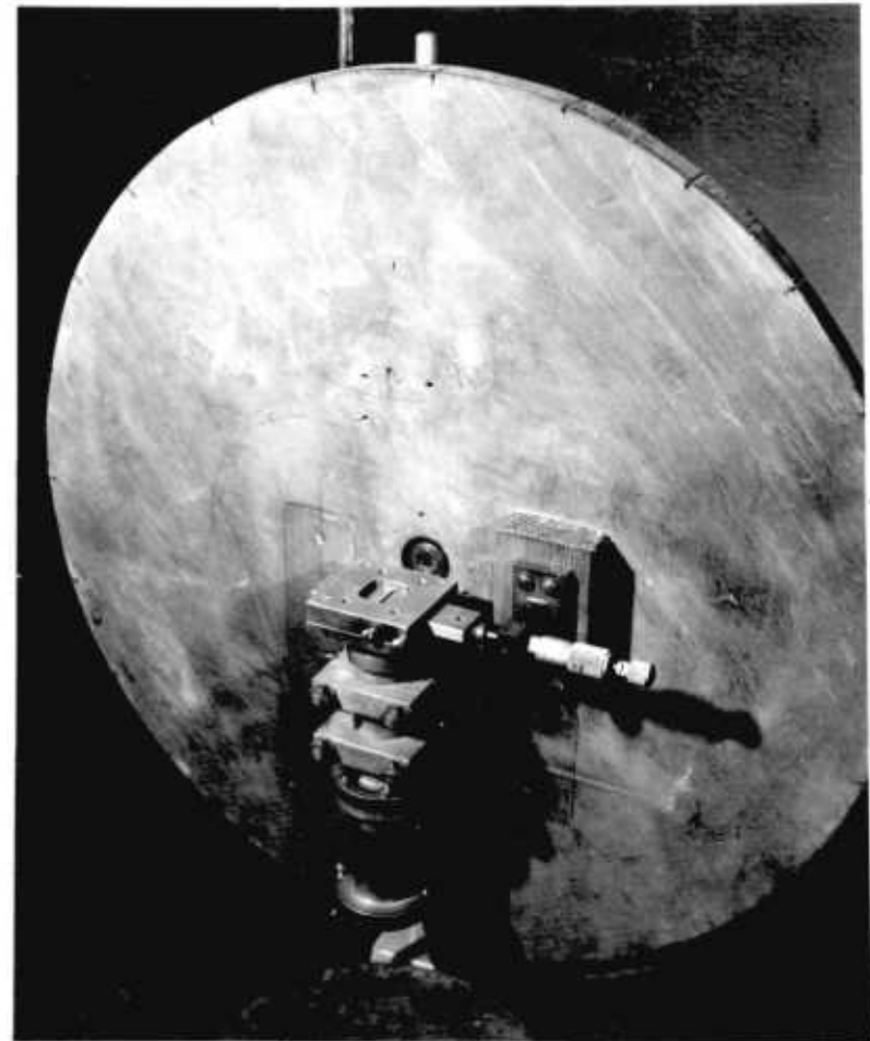
Fig. 5.6. Flashback burner mounted on baseboard
