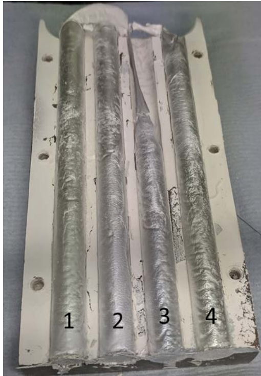
Figure 3.1 The casting sample with four cylinders in a pre-heated BN coated steel mould.
