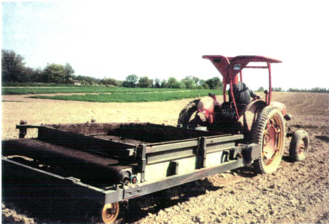
Plate 3.2 Spreading of compost prior to field experiments (spreader designed by technicians at Wye College Agricultural Engineering Workshop).
