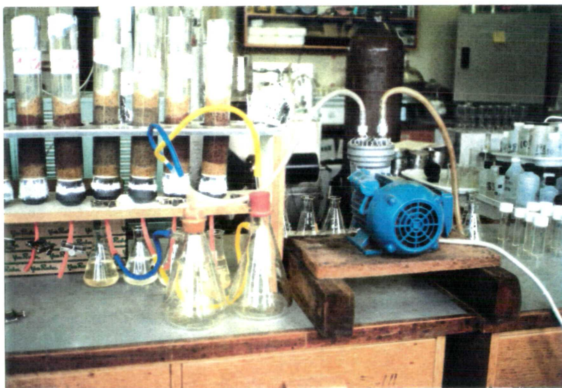
Plate 8.2 Vacuuming to remove excess solution from soil in leaching tubes. Drainage stems are then closed and tops covered to avoid moisture loss.
