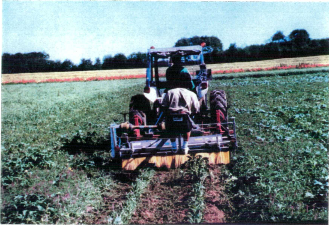
Plate 5.1 Inter-row brush weeder being used for mechanical weed control in the 1994 Field A experiment
