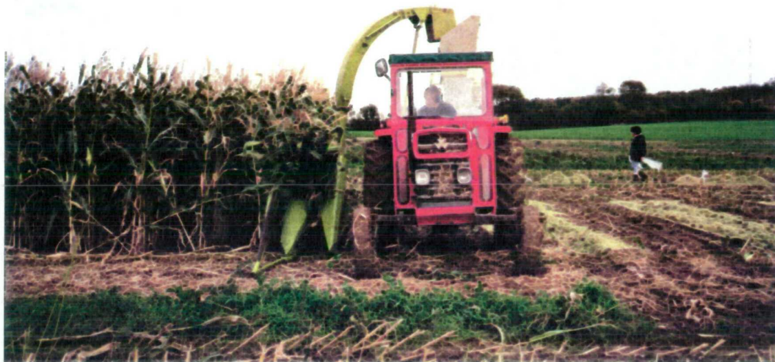
Plate 3.3 Single-row forage maize harvester used in all field experiments. Maize plants in rows were chopped and collected in a container (Plate 3.4).
