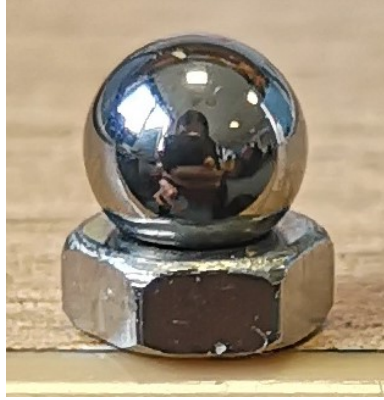
Figure 5.17: Photo of the 5 mm diameter, grade 10, tungsten carbide ball-bearings used as a novel “knife”-edge for penumbral imaging in this project.
