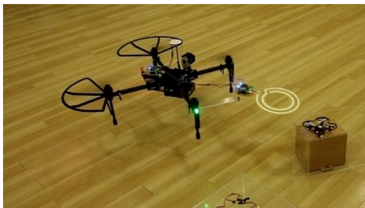
Figure 7.12: Photograph of a DJI Matrice 100 drone with an on-board HF-IPT transmitter.
