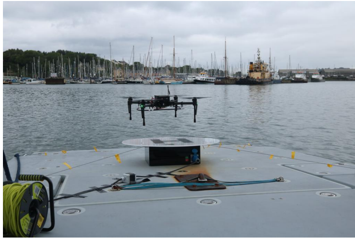
Figure 7.13: Photograph of the wirelessly charged drone taking off from the developed transmitter platform. The photograph was taken in the Maritime Autonomous Systems Trials and Evaluation Centre located at Turnchapel Wharf, Plymouth, UK, on the 11th of June 2019.
