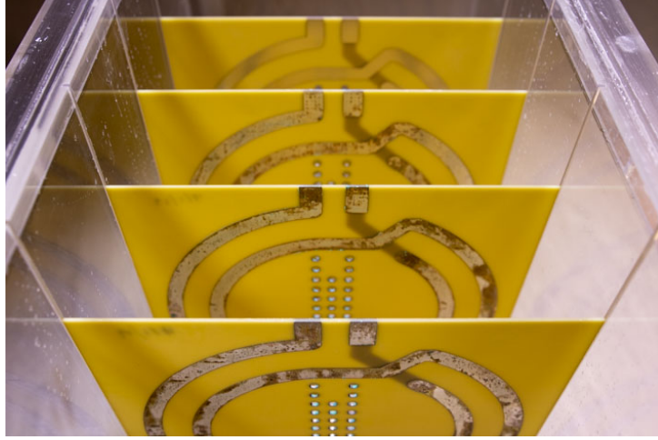
Figure 4.19: Photograph of the gradually corroded coils in the corrosion chamber.
