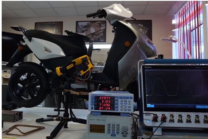
Figure 7.21: Photograph of the 600 W wireless charging experiment of the on-board battery of a Govecs S2.4 Electric Scooter.
