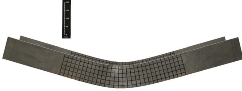
Figure 18: Typical failure mode for minor axis bending, shown for specimen I-220×110×6×10 (B16).
