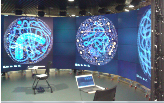
Figure 1: Partial view of the KPMG Data Observatory at the Data Science Institute, Imperial College London. Its 64 46' screens create a 313 degree immersive space with a total resolution of 132M pixels. Users can walk in, and collaboratively explore data presented in different ways (charts, maps, animations, graphs...). The image shows Bitcoin transaction being displayed [8].
