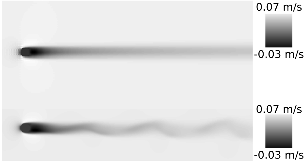
Figure 5.10: Visual comparison of instantaneous axial velocity field at Re = 300 on the two grids: coarse ( top ) and fine ( bottom ). Maximum positive velocities are shown in white, while maximum negative velocities are black.
