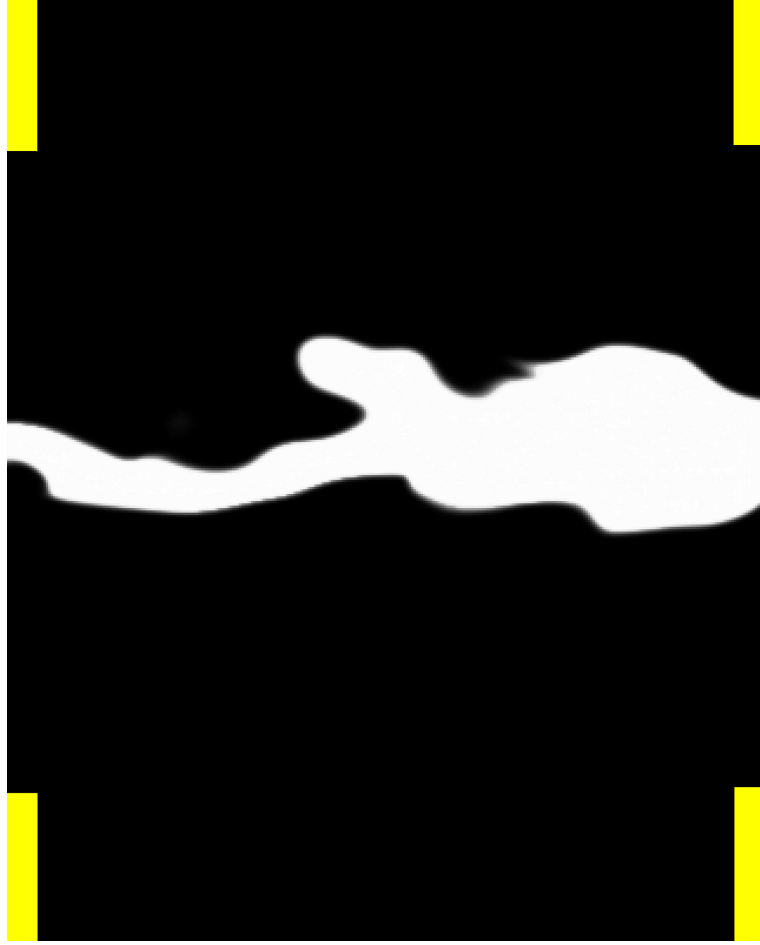
Figure 5.27: Visualisation of an instantaneous progress variable field between the nozzles for a bulk velocity U_b = 4 m/s, \Delta = 0.1 mm and T_f = 2 . Burnt regions are shown in white, while unburnt regions are shown in black.
