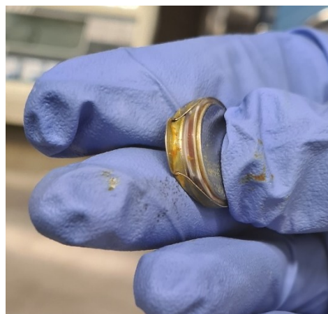
Figure 37: Casing damage of a coin-cell due to misalignment when crimping
