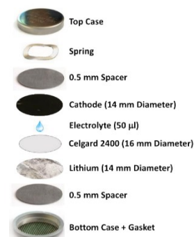
Figure 2: Coin-cell schematic diagram, taken from [37]
