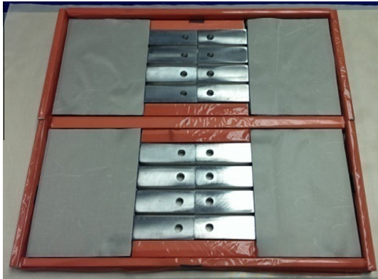
Fig. 4. Specimens ready to be cured after laying up.
