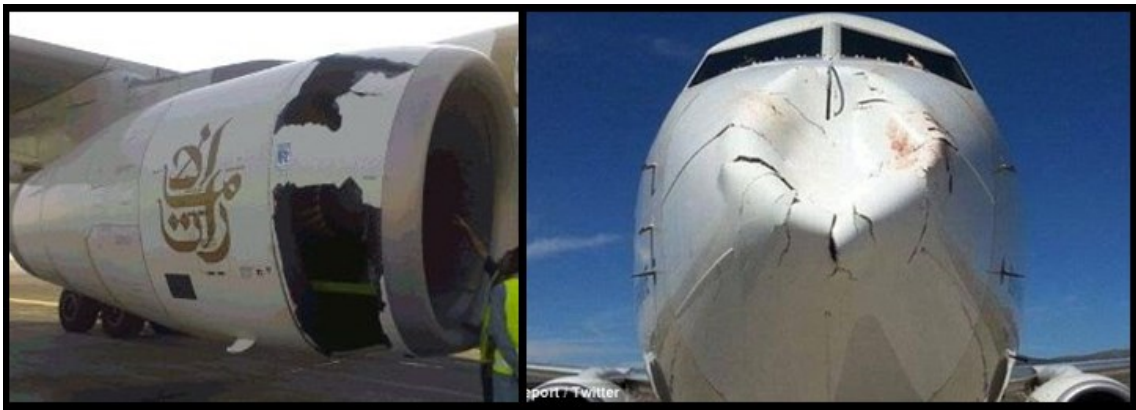
Figure 1-4. Illustration of damage on an aircraft’s composite sandwich structures. Left: Emirates airbus rolls royce engine cowling went to pieces happened on 18 Oct 2006 [11]; Right: The nose cone was flattened by a sever bird strike as the plane landed at Nevşehir in Turkey [12].
