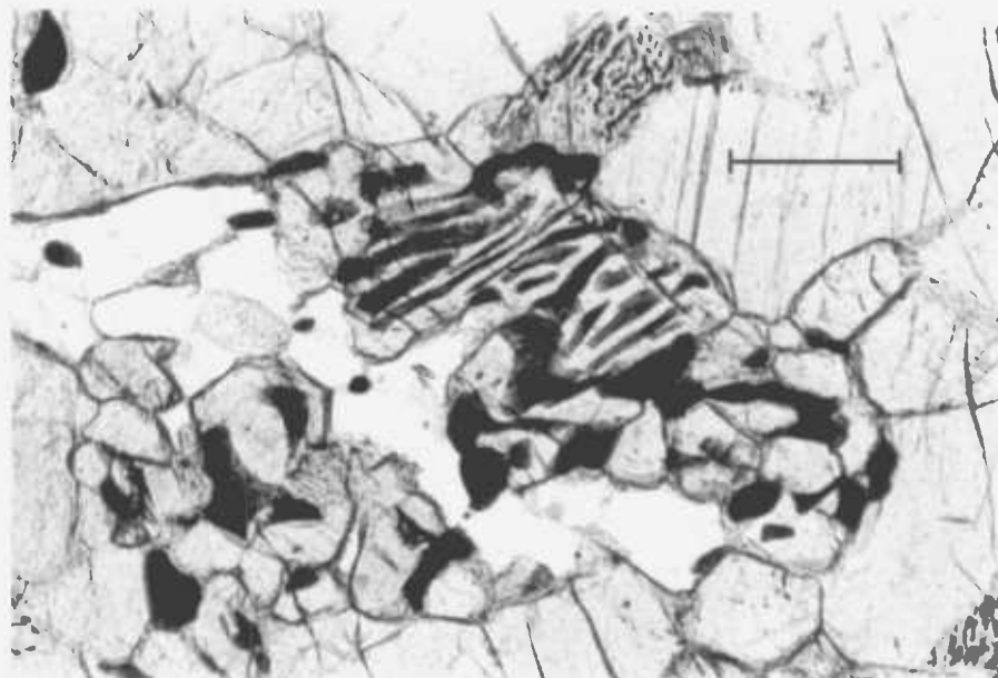
Plate 2.16 An orthopyroxene (grey)-spinel (dark grey-black)-plagioclase (white) symplectite (after garnet) from sample 85. The spinel is present as amoeboid lobes within the orthopyroxene. Coarse, relict orthopyroxenes and clinopyroxenes surround the fine grained symplectite area. Scale bar is 0.25mm. Plane-polarised light.
