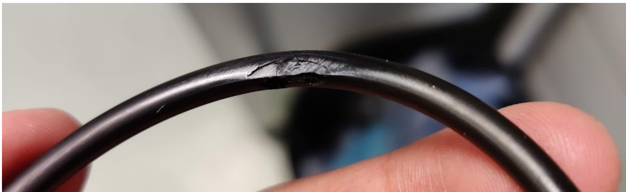
Figure 4.12: Damaged HCL O-ring due to a sputtered glowing-hot Nd flake landing nearby.
