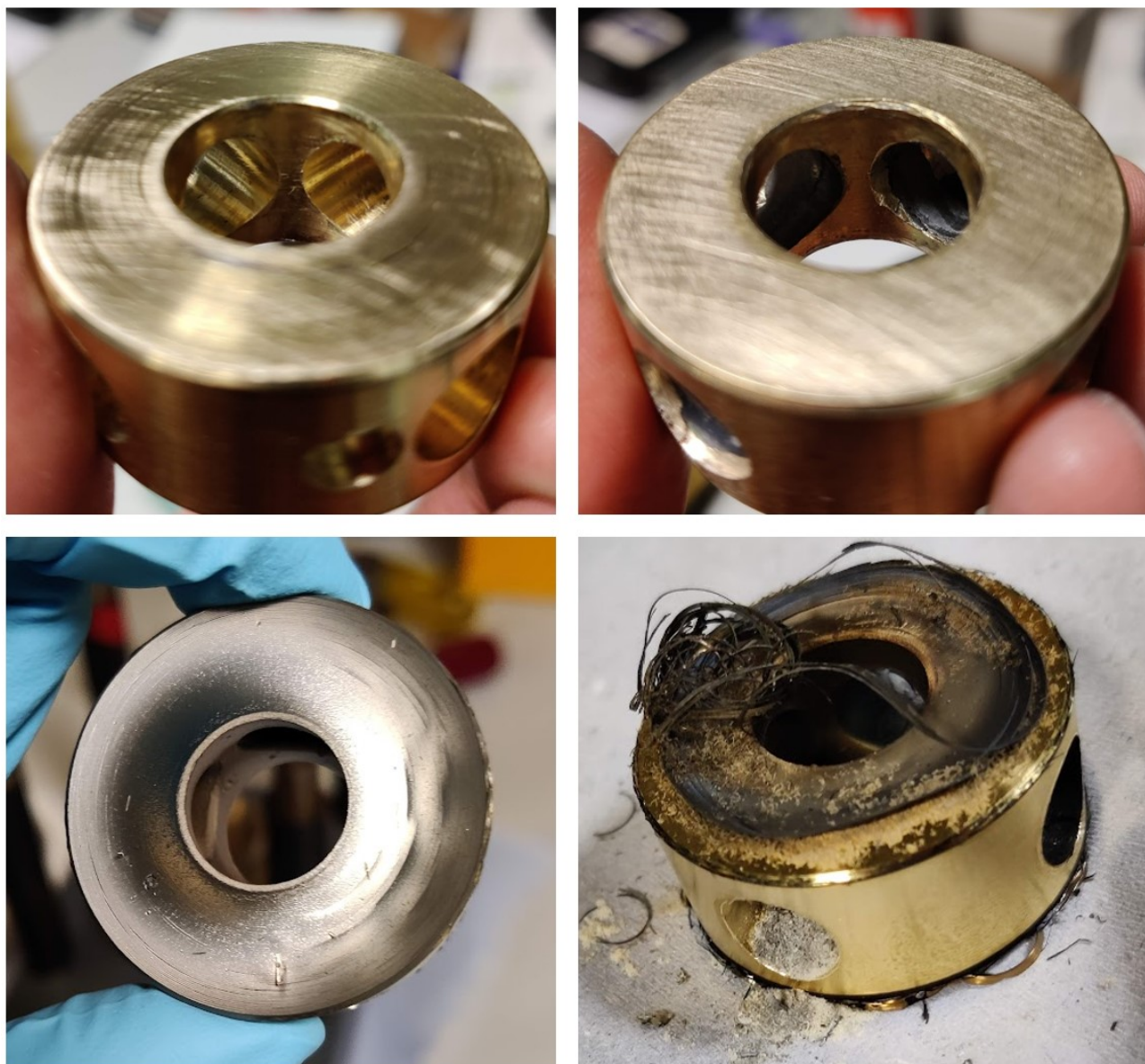
Figure 4.11: Photographs of PDL anode rings: (top-left) new anode ring and cleaned after a single use; (top-right) worn anode ring and cleaned after multiple uses, chipped corners are visible, Nd coating remaining within the holes were not removable by force, (bottom-left) anode ring taken out of the PDL immediately after an experiment, fully coated with Nd, and (bottom-right) anode ring taken out of the PDL after an experiment, but rested under the atmosphere for two days, very thin coatings of Nd were reduced to the light grey Nd oxide dust visible at the bottom hole, slightly thicker layers near the circumference at the top has reduced into curled flakes of dark grey colour.
