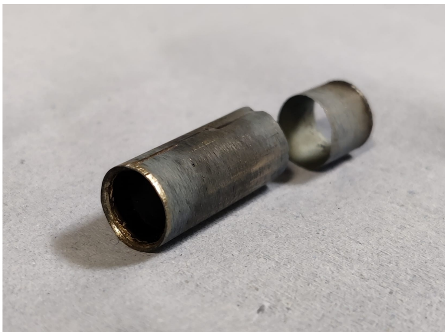
Figure 4.9: Photograph of the depleted Nd hollow cathode, where the broken section was the thinnest.
