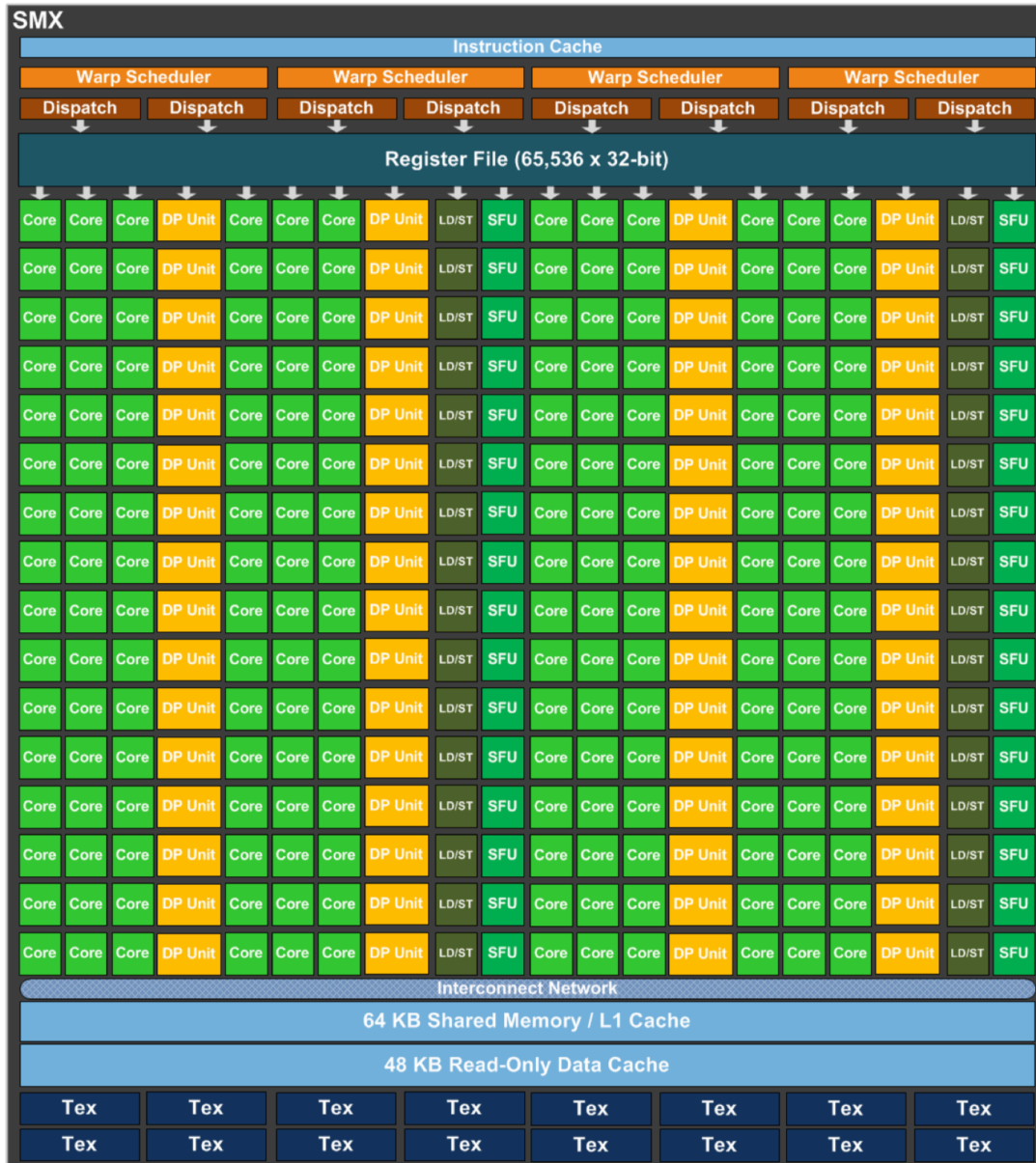
Figure 2.7: Streaming Multiprocessor (SMX) of the GK110 Kepler architecture [63]
