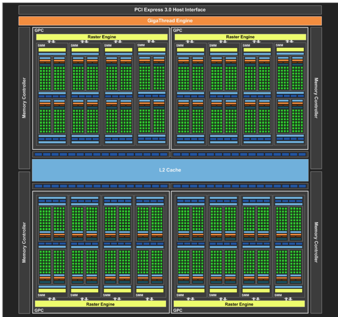
Figure 2.12: Full-chip block diagram of GM204 chipset, Maxwell architecture [64].
