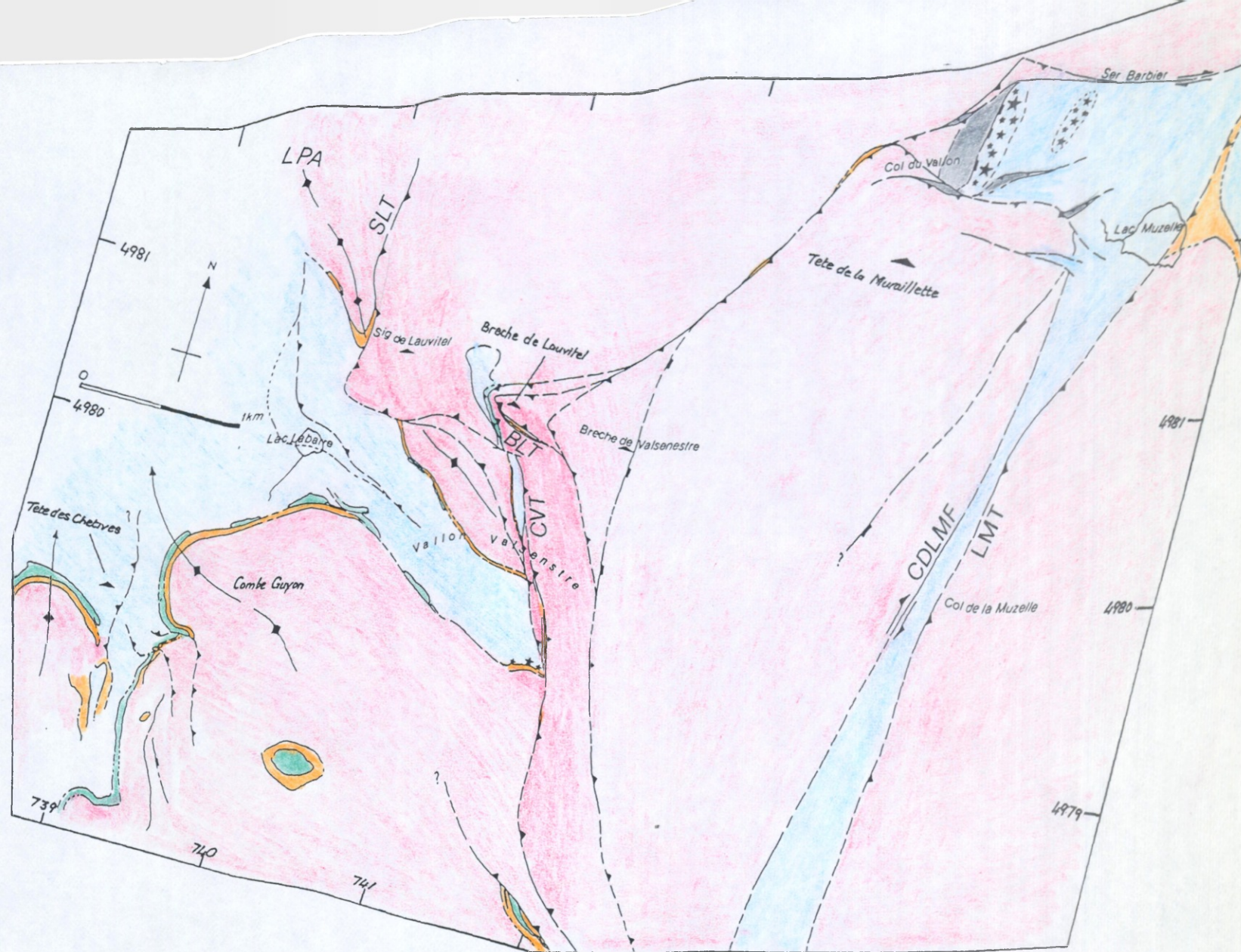
Figure 2.3.5: Simplified structural map of the Vallon Valsenestre area (location and legend indicated in Figs. 1.7 & 1.8). LMT-Lower Muzelle thrust, CDLMF-Col de la Muzelle fault, BLT-Breche de Lauvitel thrust, CVT-Cabane du Vallon thrust, SLT-Signal de Lauvitel thrust, LPA-La Paletas anticline. Based on mapping by the author.
