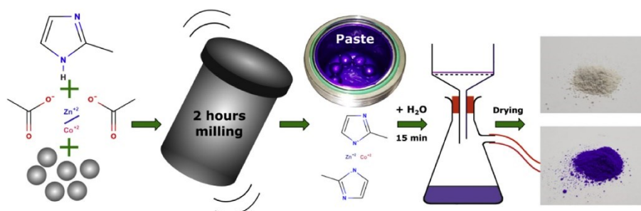
Figure 1.10 Example of preparing Co-doped ZIF precursor by ball milling method. [Printed with permission from Ref 129 . Copyright © 2019, Elsevier Ltd.]
