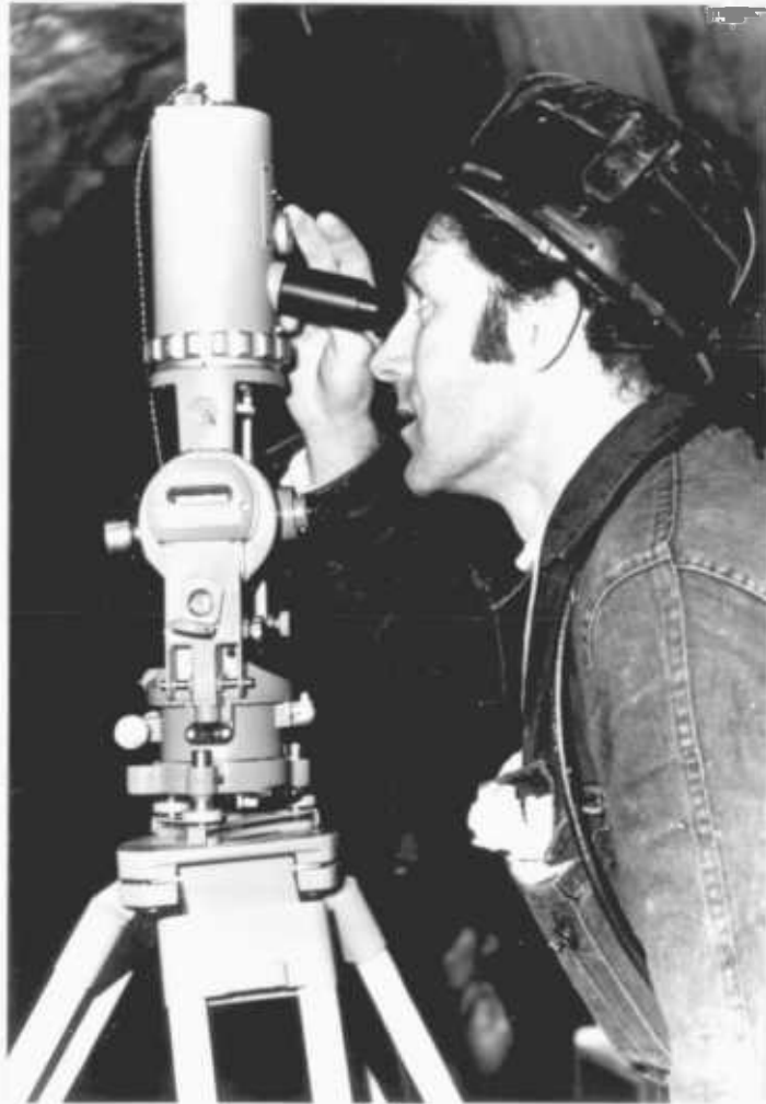
Plate 6 - An Underground Observation with the R.S.M./Wild Modified G.A.K.-1
