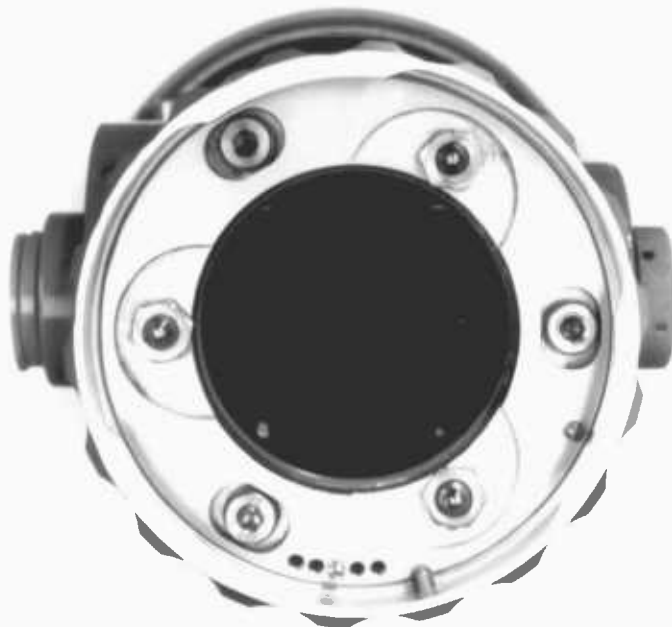
Plate 2 Three Pin Locating System in the "Bridge" of the Wild G.A.K.-1
