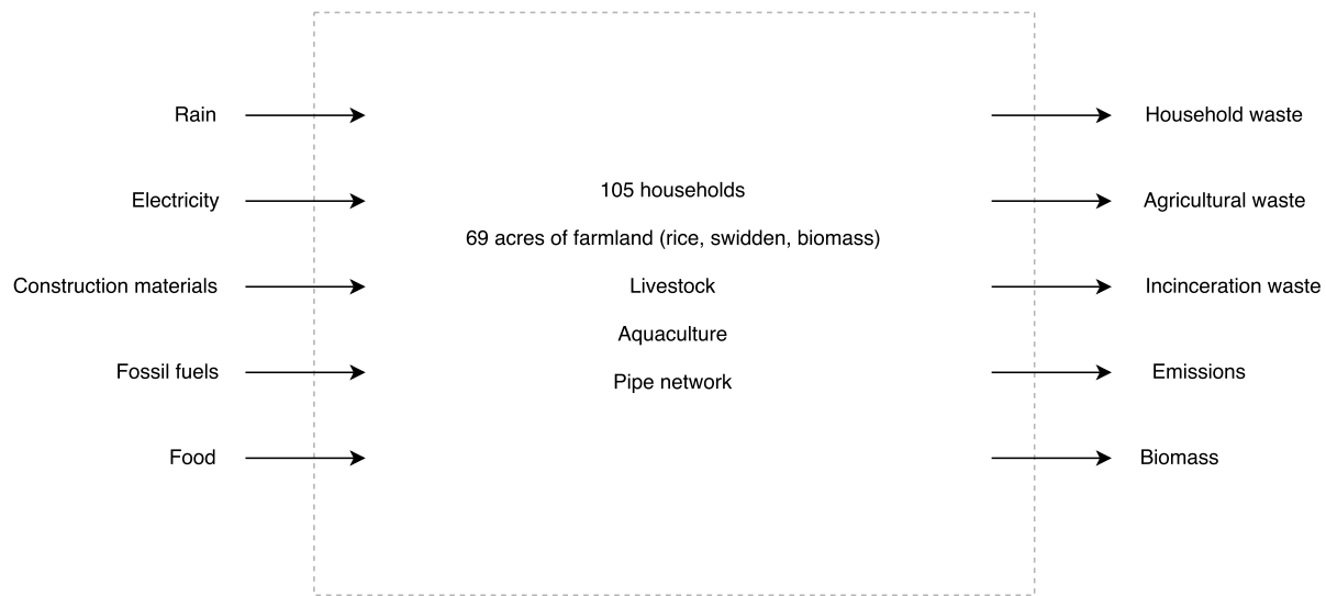
Figure 5.1: A summary of the resources and processes in Tat's metabolism. The dotted line represents the boundary across which Tat imports and exports resources which are managed internally.
