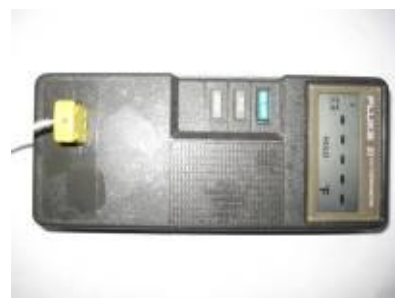
Figure 3.17 A Fluke thermocouple module for an oil temperature measurement
