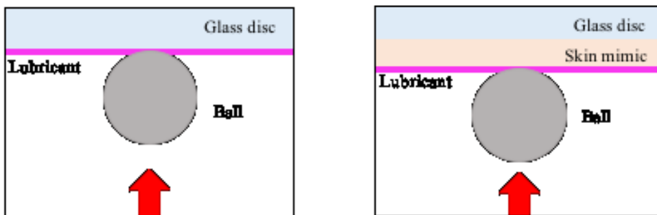
Figure 6.9: Calibration setup for (a) glass disc (b) silicone elastomer disc
