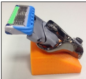
Figure 7.3: Razor cartridge mount for LIF tests
