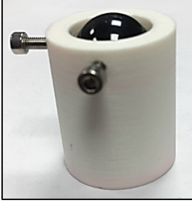
Figure 6.4: Sample spacer with fixing screws
