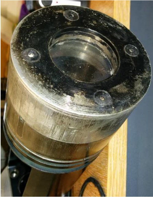
Figure 2.2 Actual view of the Ricardo Hydra optical piston (C. K. H. Hong, 2015).
