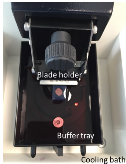
Figure 6.5 The set-up of the vibratome.
