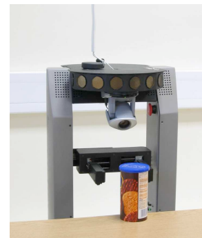
Fig. 2: A PeopleBot moves in to grasp an object. The Peoplebot’s grippers do not extend, so it can only grasp objects at the very edge of a table.
