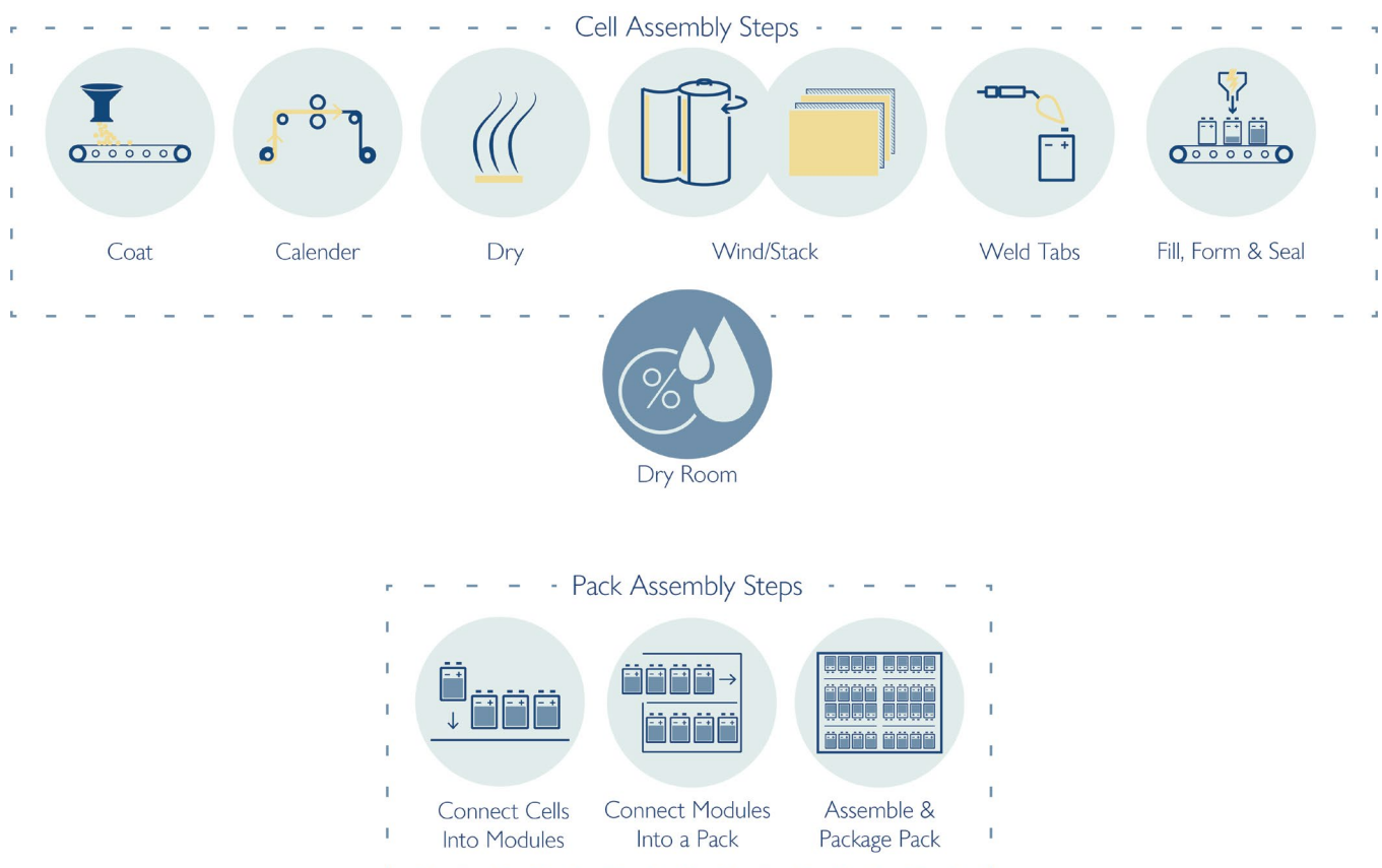
Figure 8. Cell and pack assembly process. Cell assembly is usually conducted in a dry room, due to the sensitivity of Li compounds to humidity.
