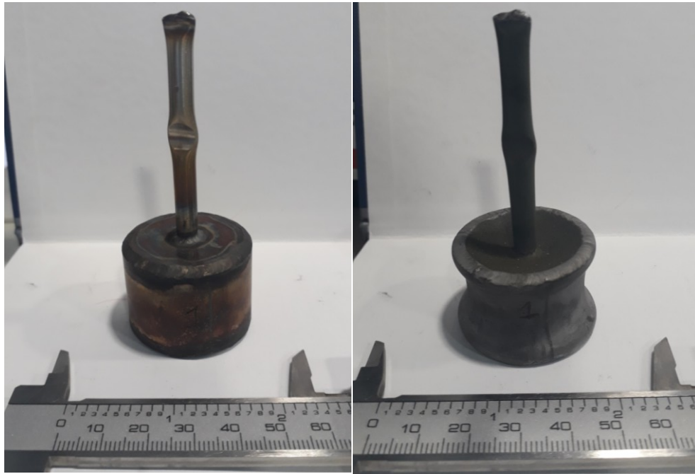
Figure 2.2 Photos of HIP canister before (left) and after (right) HIPing. The unit of calliper is mm. Provided by Dr. Laura Gardner, the University of Sheffield.
