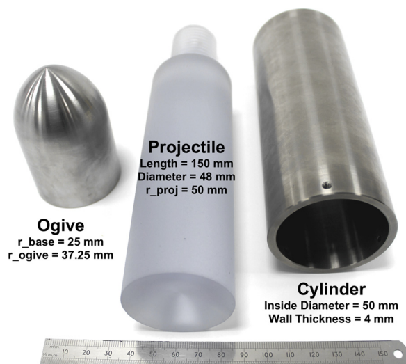
FIG. 5. Left to right: Ogive, projectile, and Ti-6Al-4V cylinder as used in Sec. IV B. Threaded section at the top of the projectile is used to attach it to the sabot.
