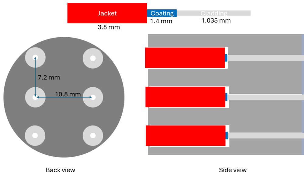
Figure 68 Back and side view of the second iteration fibre housing unit with fibre.
