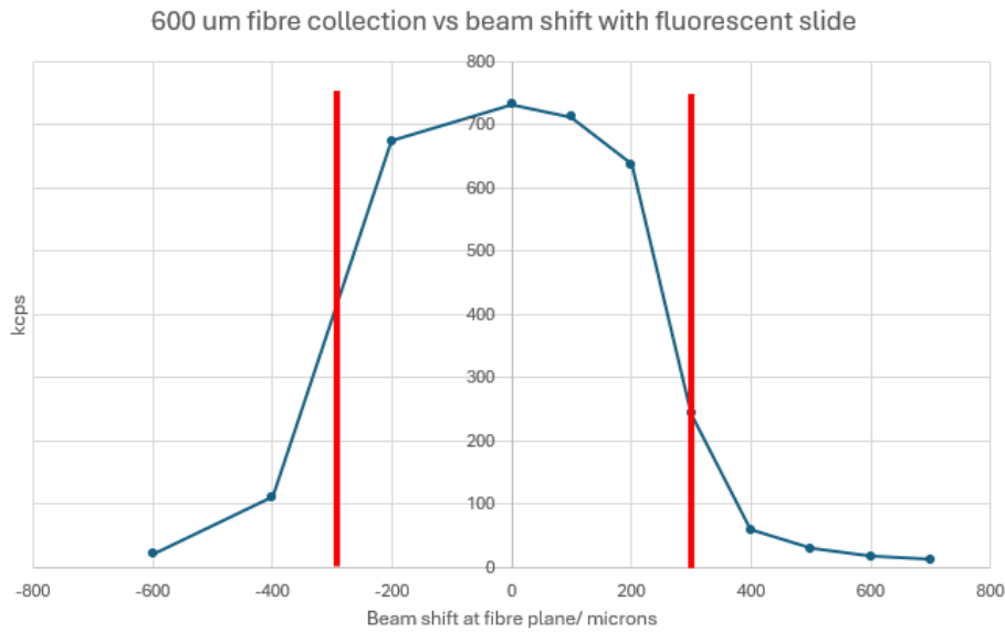
Figure 53 PMT counts as a function of beam shift at fibre plane using a fluorescent slide. Red lines indicate fibre diameter. FWHM of the beam at the fibre plane is \sim 30 \mu\text{m} .
