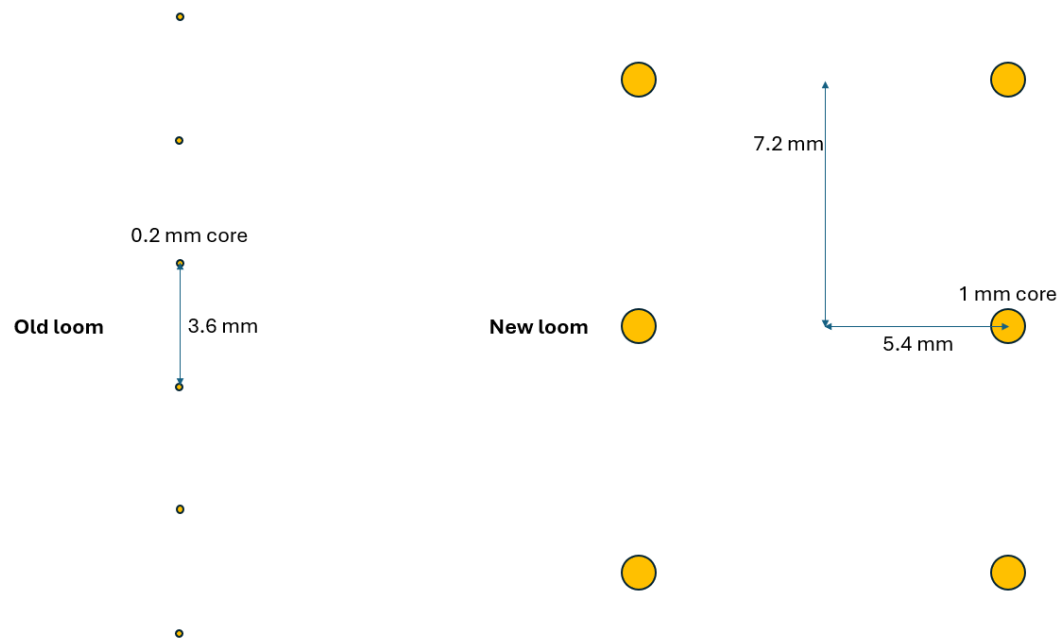
Figure 67 Comparison between old and new fibre looms geometries. (To scale)
