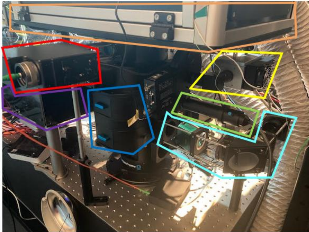
Figure 27 Photograph of openFrame microscope in a later configuration showing autofocus unit (red), incubator (orange), NDD (yellow), single photon illuminator (green), phase imaging path (cyan), slider layers (blue) and multibeam multiphoton excitation breadboard (purple).
