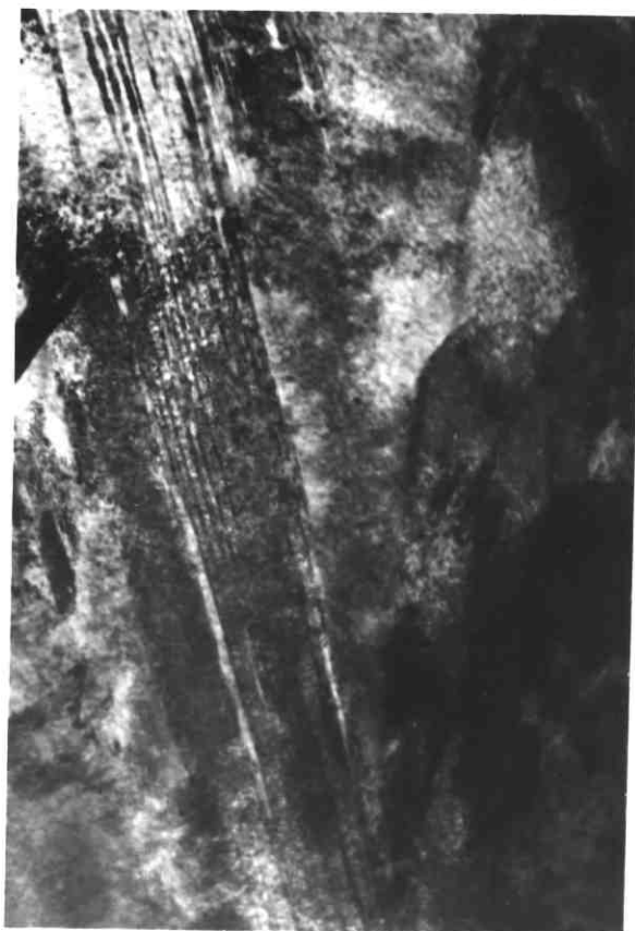
Plate18- Fine internally twinned martensite in as-quenched En24 steel after 10 5 s at 750°C+WQ
