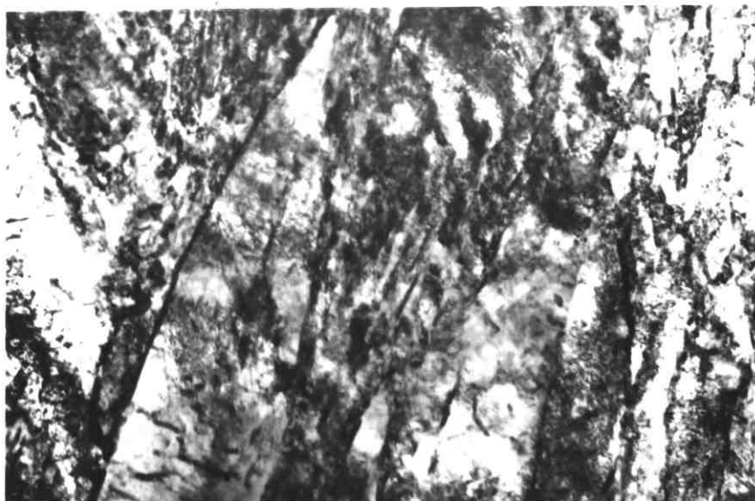
Plate8-0Q.En24 steel,5s at 720°C+WQ
