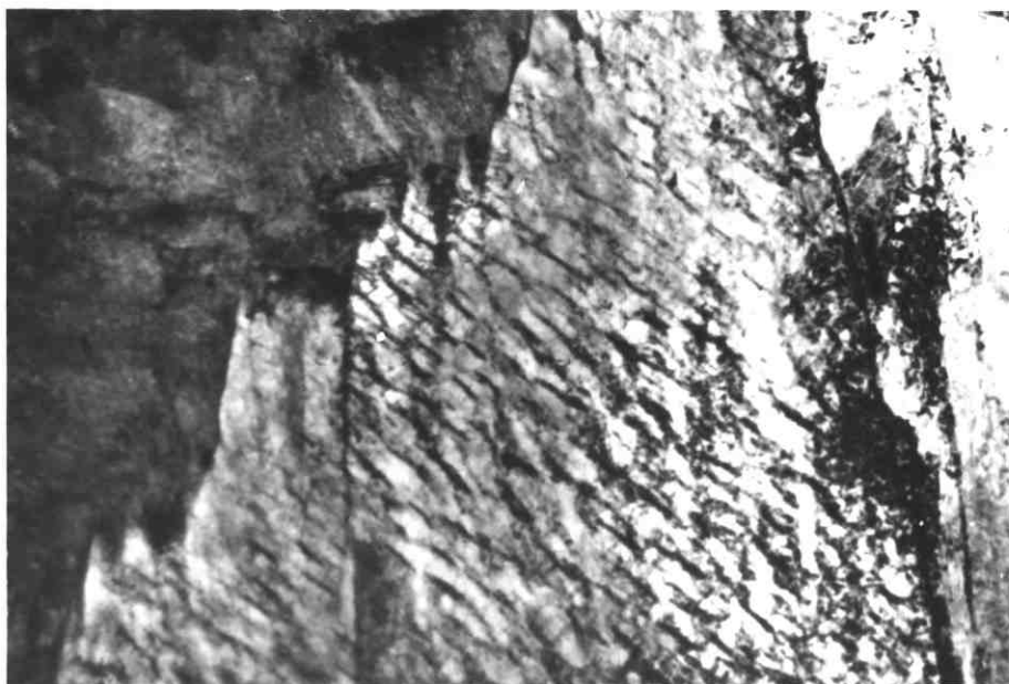
Plate 5- Autotempered martensite in as-quenched \text{---}0.2\mu\text{---} En24 steel T.E.M.
