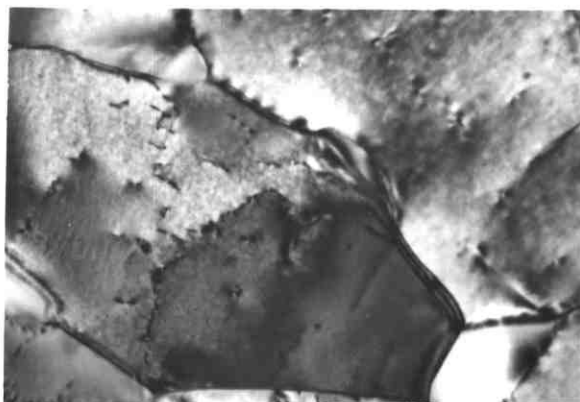
6-b-Recrystallized \alpha grains |—0.2 \mu —|
