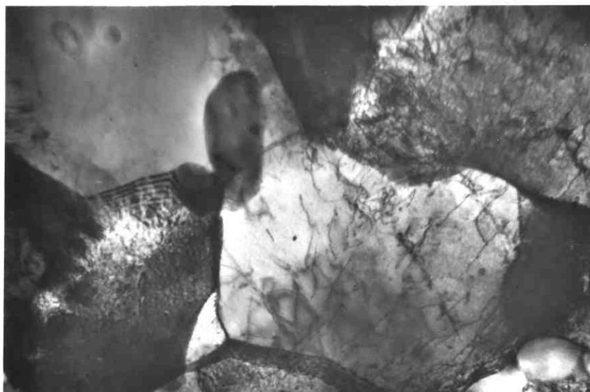
Plate9-0Q.En24 steel,10 5 s at 720°C+WQ
