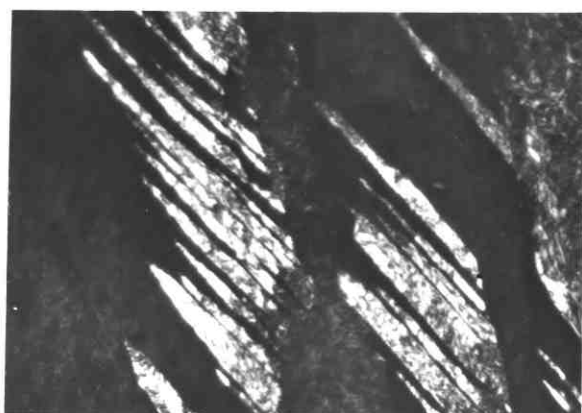
Plate 3-b-High resolution dark field of twins
