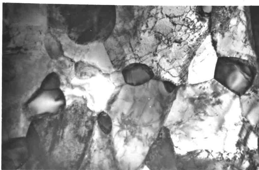
Plate10-QT.En24 steel,10 5 s at 720°C+WQ
