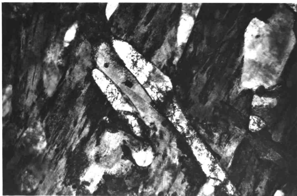
Plate14-OQ.En24 steel, heated for 10^4 s at 735°C (S.B.) + WQ
