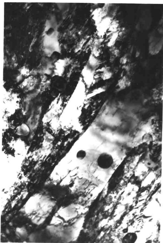
Plate17-Lamellar structure of ferrite+martensite and equiaxed particles in 0Q.En24 held for 10 3 s at 750°C+WQ
