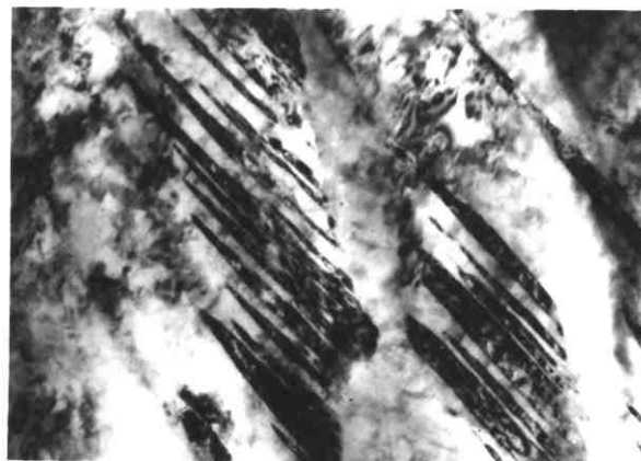
Plate3-a-Bright field—0.2μ— showing internal twins x100K
