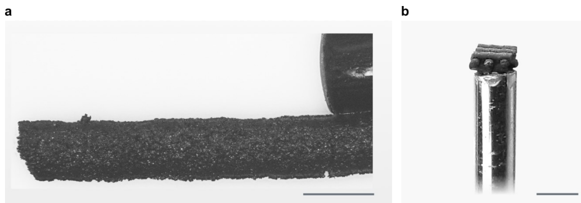
Figure 2.9: (a) Printed graphene sample attached to a graphite rod (0.5 mm in diameter) for X-ray tomography (scale bar 500 \mu\text{m} ); (b) Printed zinc sample attached to an aluminium rod for X-ray tomography (scale bar 2.5 mm).
