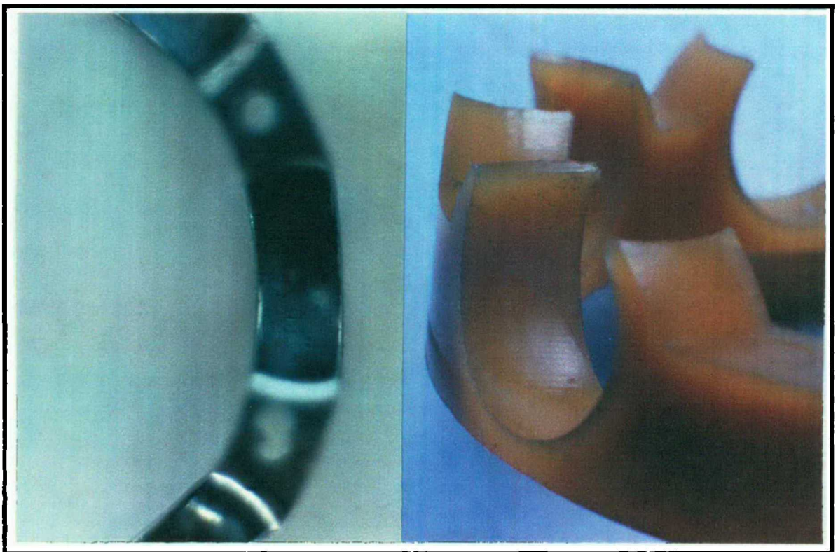
Figure 7.24. Photograph of wear marks on a plastic and steel cages from bearings run with 6\mu\text{m} silicon carbide abrasive.
