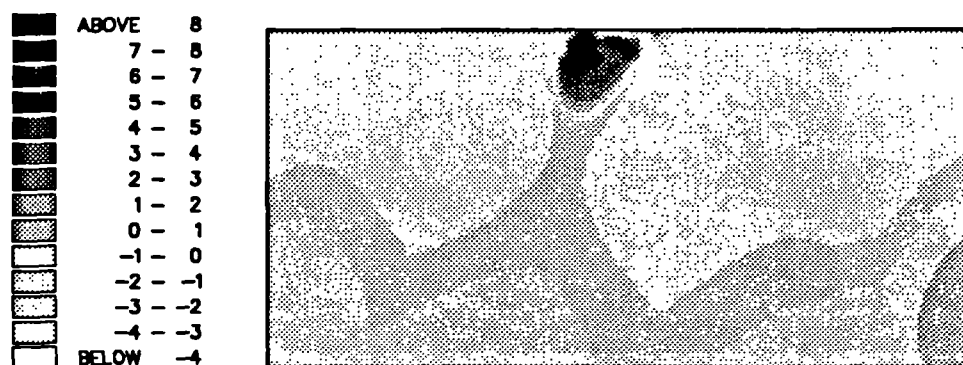
Figure 5.17. Fatigue life risk map for a surface containing a 10 slope degree asperity, residual stresses not included, friction coefficient 0.1.
