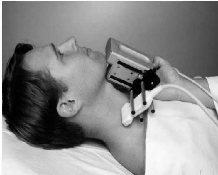
Figure 3- 4 A mechanical linear scanner mechanism used to acquire 3D ultrasound images of the carotid artery (Fenster et al., 2004).
