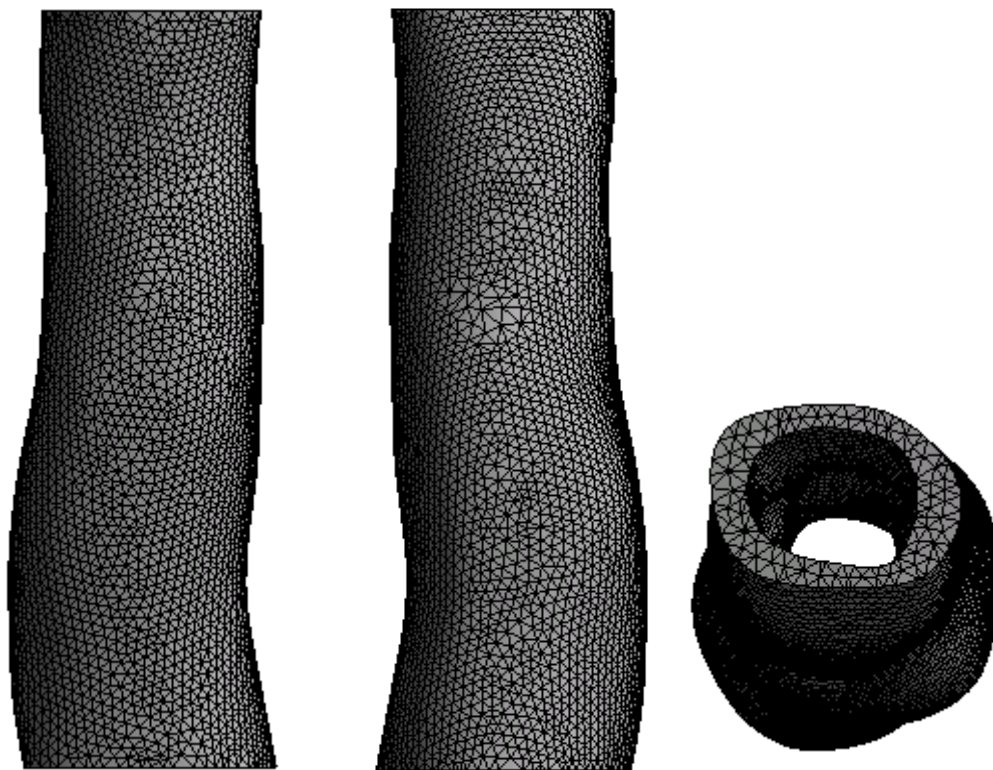
Figure 4- 18 Spatial discretization of the carotid artery in patient 1: Frontal view (left); Lateral view (middle); Top view (right)
