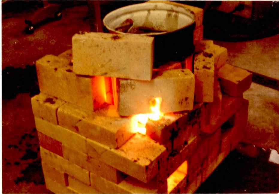
Figure 6.1 Reacting Slag Pouring From Lanced Firebrick
