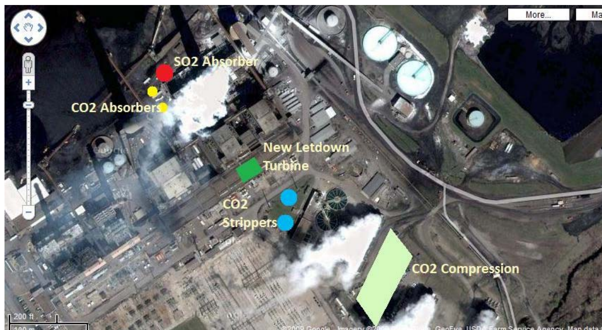
Figure 4-10 US Conesville proposed retrofit unit
