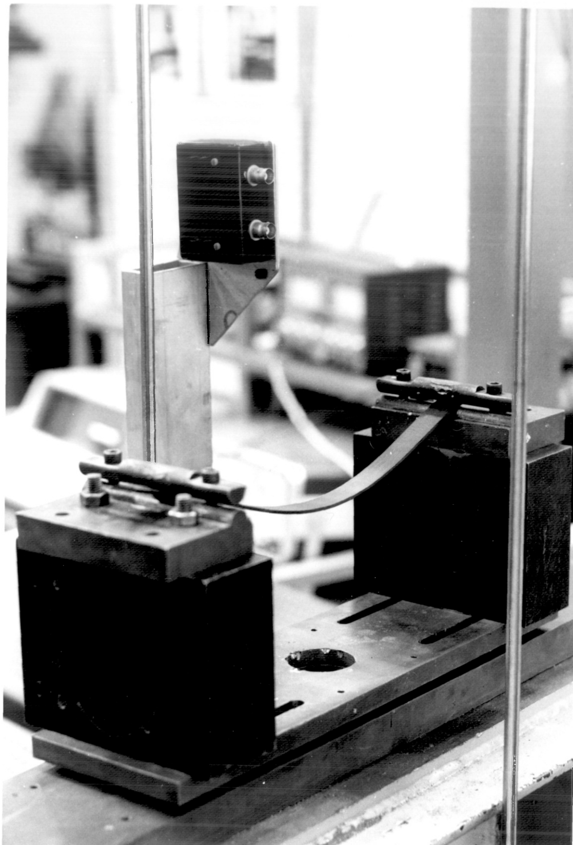
PHOTO. (4.7) - Composite beam locked in deflected position
