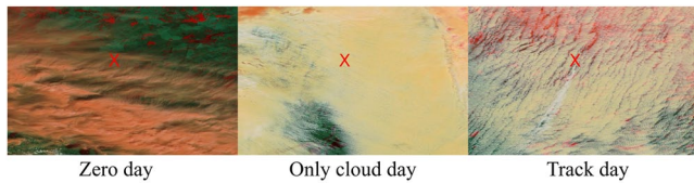
Figure 1. Classification of days. Zero day means there is either no cloud or no suitable cloud. Only cloud day means a suitable cloud exists where a pollution track could form, but no such track is visible. Track day means that a pollution track has formed in a suitable cloud. These images show the area surrounding Thompson, Canada, a known pollution hot-spot, which is marked with a red “x.” Green and red on the leftmost image signify vegetation and ice/snow, respectively. There is an ice cloud on this image, in which pollution tracks rarely form. Therefore, it is classified as a 0 day. The pollution track is the brighter part of the cloud in the rightmost image, which flows out from Thompson as from a point source.
