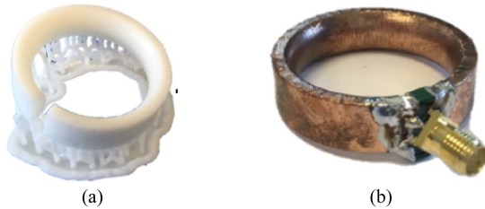
Fig. 5. Prototype of the single-turn high-Q coil. (a) Three-dimensional printed coil frame. (b) Copper-plated coil with compensation capacitors and connector [12]. (IEEE Copyright).
