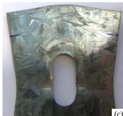
Fig. 2 Typical failure modes of bolted connections: (a) shear-out failure; (b) bearing failure; (c) net section failure [9]
